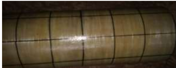
Fig 10 Grid formation for NDT(ultrasonic test)
