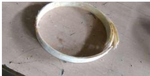
Fig 16 Delamination of fiber layers from fabric
